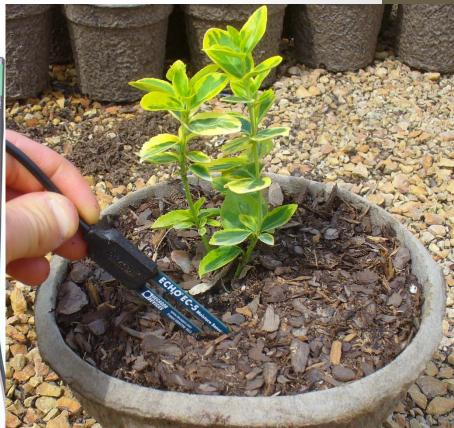
Substrate volumetric moisture content determined with Theta probes or Decagon 10HS sensors via a Campbell datalogger programmed to calculate
