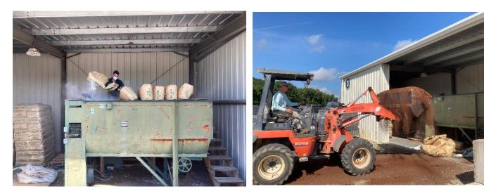
**Figure 9.** (left) Loading course perlite into  $3.8 \text{ m}^3$  (5 yd<sup>3</sup>) paddle mixer, and (right) loading bulk aged loblolly pine bark into the paddle mixer.
