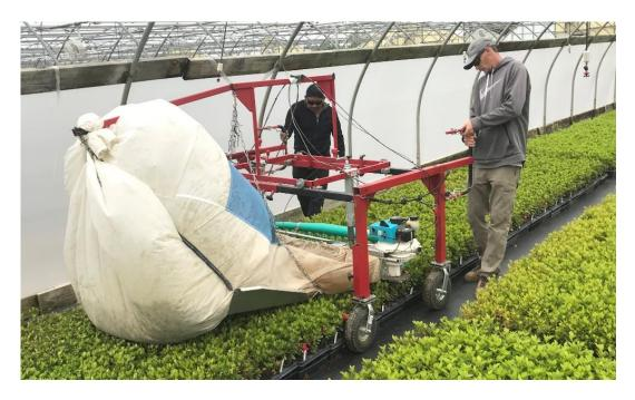
Figure 26. Gas powered sickle bar pruning machine with blower and bag attachment for uniform pruning and debris collection.
