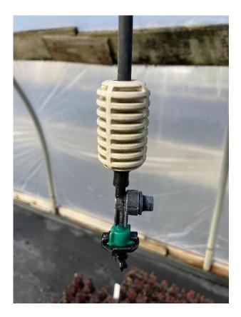
**Figure 16**. (Top, bottom left) Mini-Sprinklers are manufactured by Tavlit<sup>®</sup>. They are the 866 mini-compact sprinklers and can accommodate a variety of color-coded spinners which have different flow-rates. (Bottom right) An anti-drip device is included in the design to quickly discontinue the misting event.
