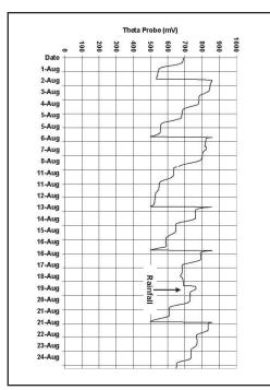
Figure 4. Theta probe output triggering irrigation.
