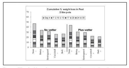
Figure 5. Effect of mulches and wetters on evaporation from pots (without plants).
