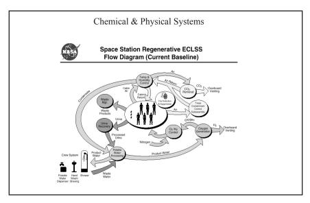
Figure 2. Chemical and physical systems for recycling and controlling water, oxygen, carbon dioxide, and nitrogen on the International Space Station.
