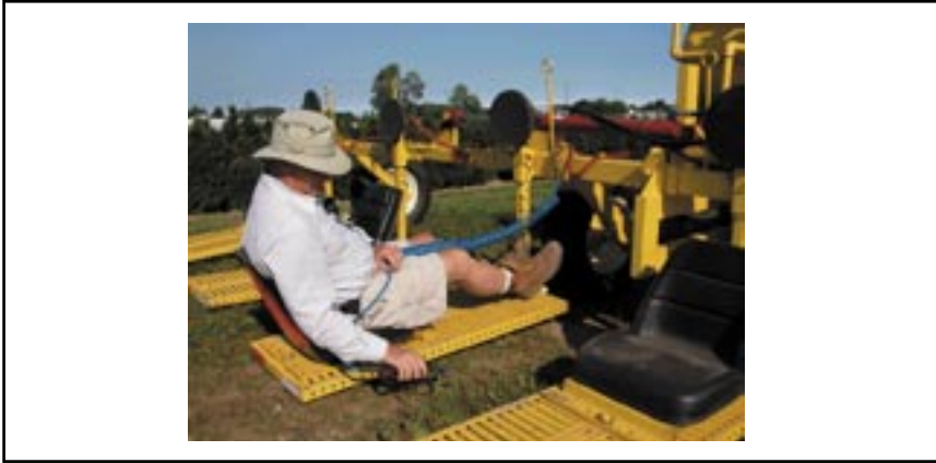
Figure 4. Piece of equipment for cutting back of budded stock in the spring.
