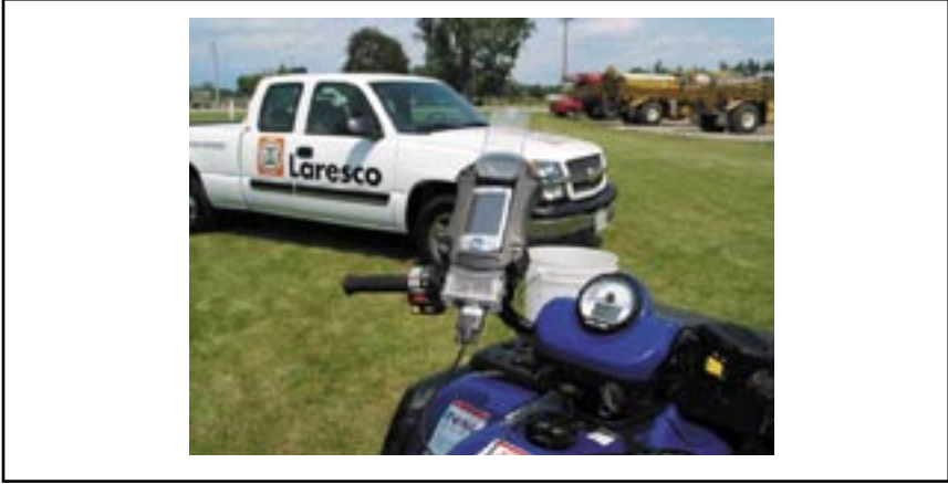
Figure 5. A satellite receiver attached to an all-terrain vehicle.
