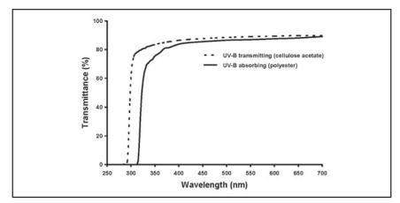
Figure 1. Comparison of UV-B-transmitting cellulose acetate with UV-B-absorbing polyester.
