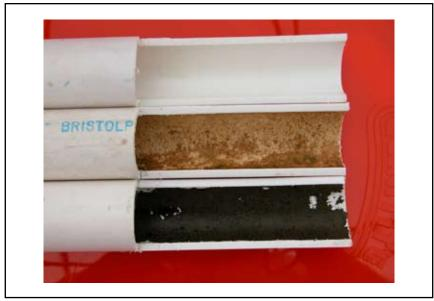
Figure 7. Longitudinally cut PVC mains; top section is new, middles section carries clear water, bottom section carries fertilizer. Note discolored biofilm layer in clear section and algae dominated layer in bottom section.
