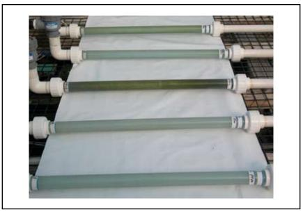
Figure 11. Clear sections of lines following continuous injection of Selectrocide with untreated control in center.
