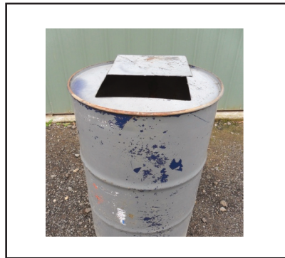
Figure 2. The flap cut from the top of the drum to adjust the amount of light entered.
