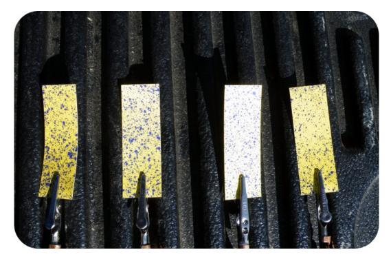
Fig. 3. Excellent coverage from Intelligent Sprayer.
