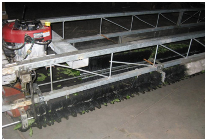
Figure 7. Prototype of 24-foot automatic trimming machine.
