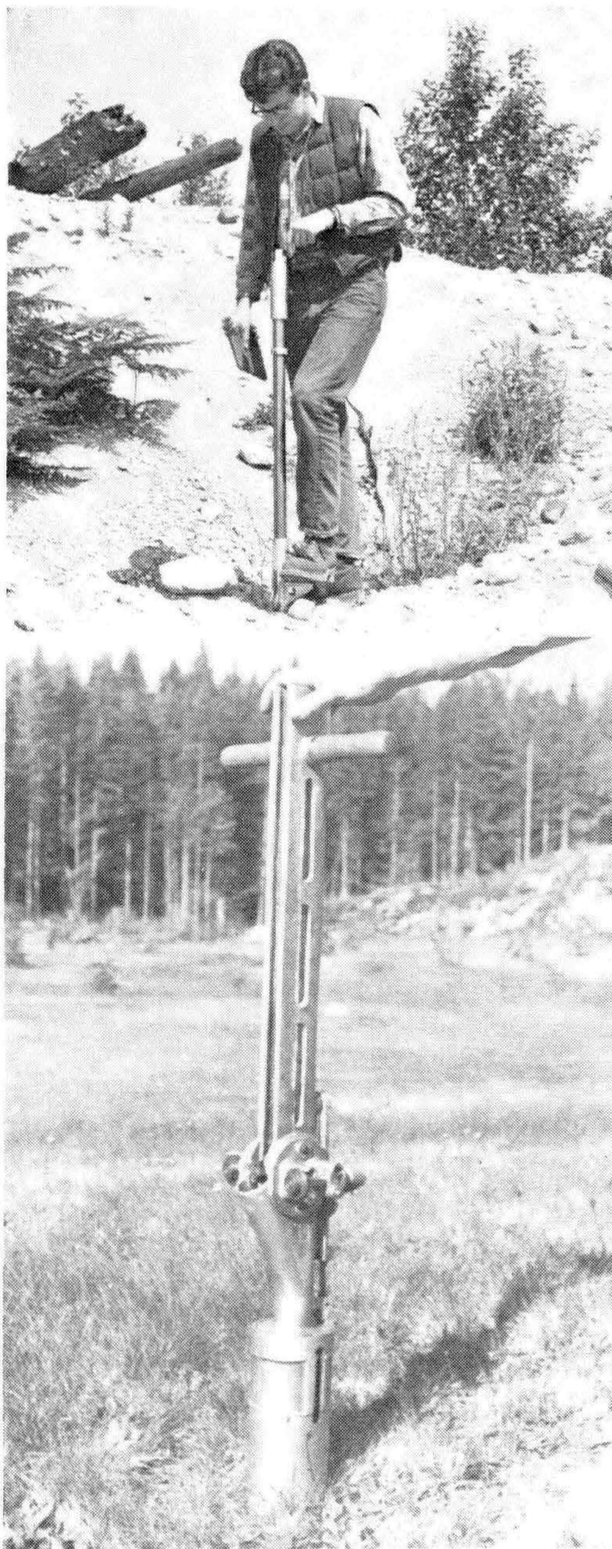
Figure 2. Planting "gun". Above. Single-shot gun in use. Below. 24-shot planting gun.
