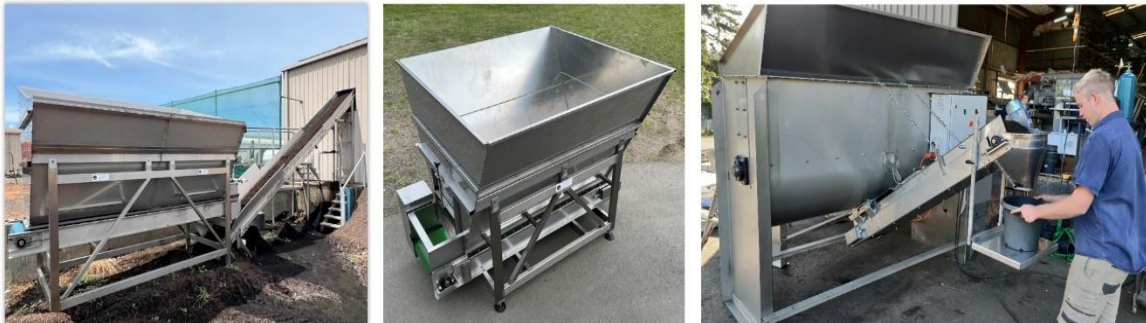
Figure 3. From left: 4Cbm Soil Storage Hopper (Left), 4Cbm Soil Storage Hopper (Middle), 2 Cubic Meter Soil Mixer with Soil Bagging Conveyor (Right).
