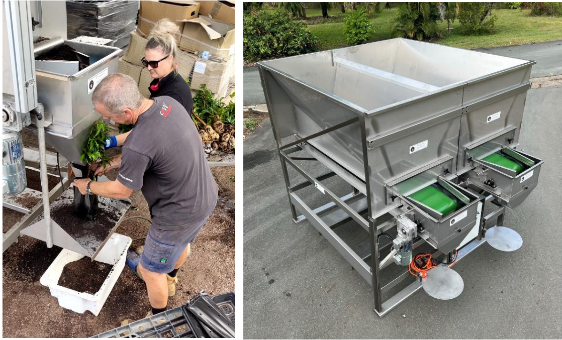
Figure 4. Pot and bag fillers are available in single and dual outlet platforms.
