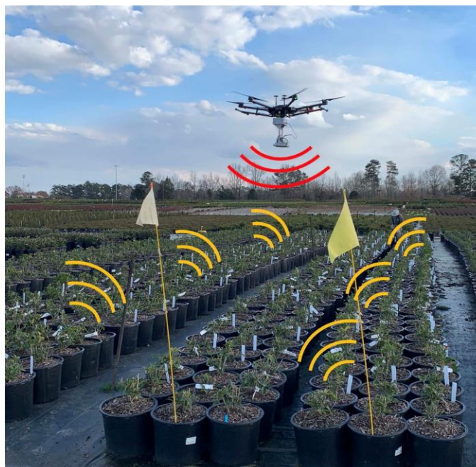
Figure 8. Merging RFID tags with drones to track and manage assets and products. A microchip and antenna make up the “tag,” which can be read by an RFID scanning device. The scanner turns the radio waves into digital data. RFID offers a major advantage over bar coding in that the scanning device does not need direct line of sight to read the tag.
