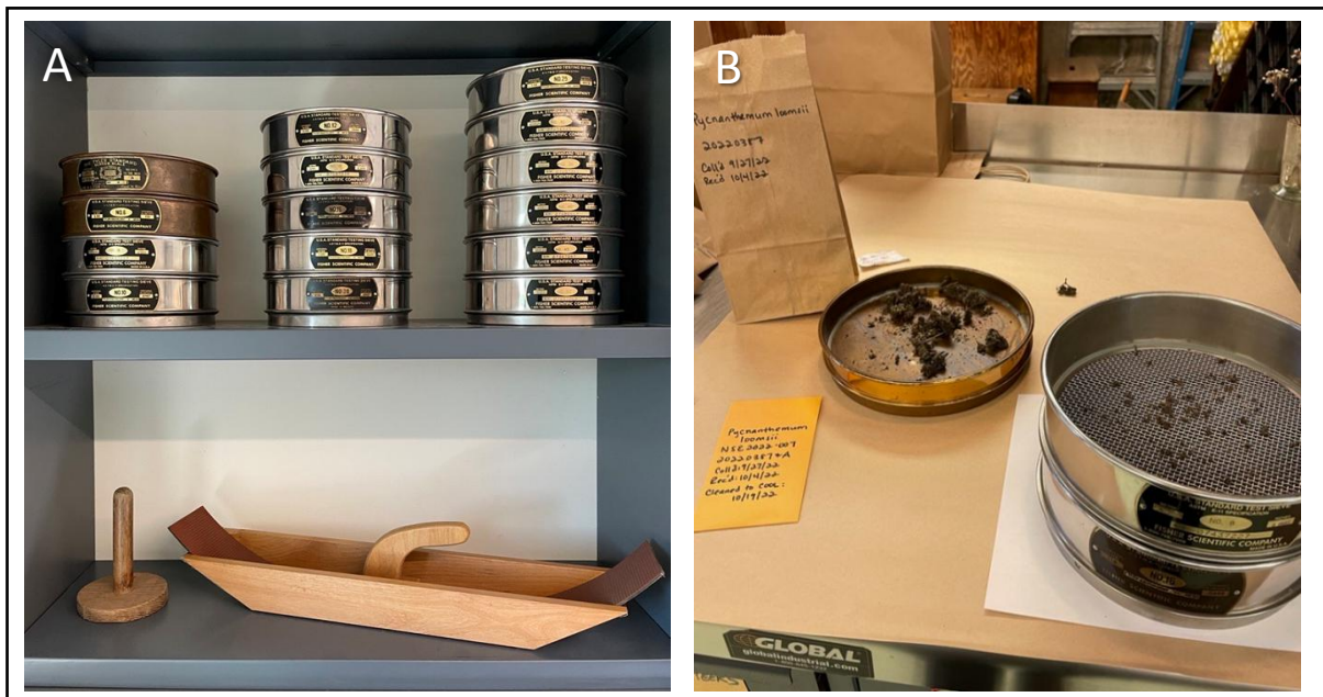
Figure 2. A) Hoffman debearder and pan sieves. B) Removing calyx parts from Pycnanthemum .
