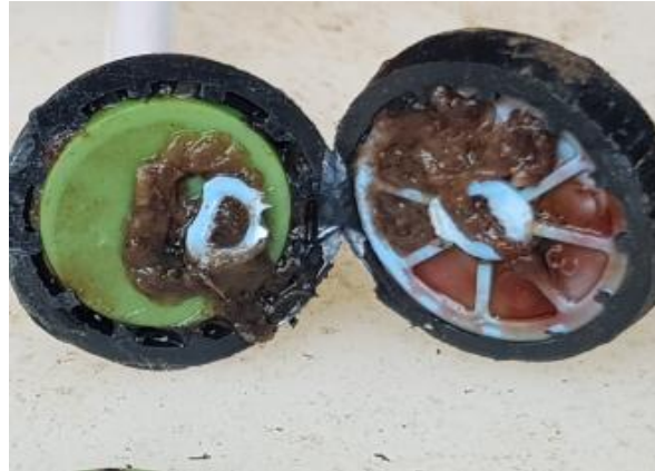
Figure 1. It is difficult to develop a single model for the qualitative composition of biofilms in irrigation systems due to factors such as geographic location, climatic conditions, type of irrigation (furrow, drip, sprinkler etc.), materials used in the construction of the irrigation system, age of the system, intensity of operation, origin of water, fertilizer addition, and system disinfection techniques. Contrasting biofilms are shown here.
